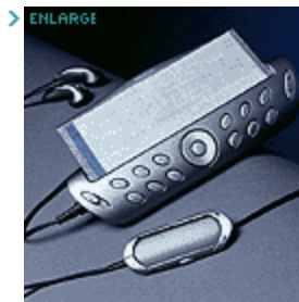
Mobile communicator for students. Design student: Anne-Mari Tornberg, 2001 Cooperating company: Nokia Ventures, Finland. This hand-held mobile aimed at the student traveller market includes e-mail, notebook and mp3 player. The physical form and roll-up screen allow rapid two-hand interaction.
